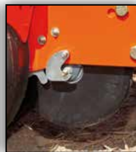
Intermediate press wheel with parking position
