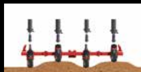
Intelligente and individual adaptation of the wheels due to the two-piece hydraulic cylinder
