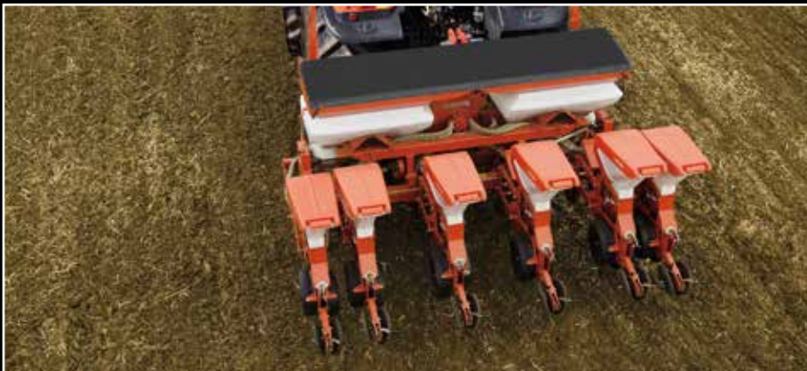
PP1450TE with 6 rows, 4.0m working width telescopic frame, 440l fertiliser hopper
