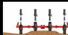
Intelligente and individual adaptation of the wheels due to the two-piece hydraulic cylinder
