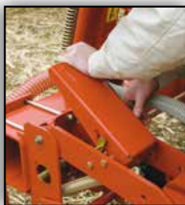
Optimal pressure adjustment by lever
