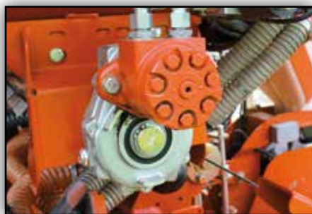
Optional electro-hydraulic drive for the fertiliser application. Fertiliser rate can be adapted even during work.
