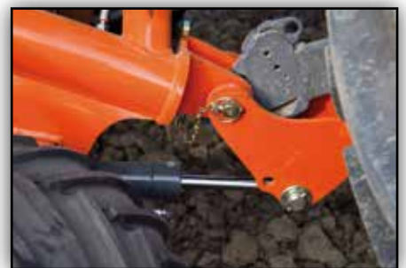
Optional hydr. frame ballasting kit
