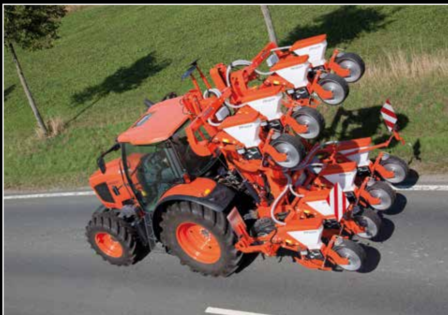
PP1600F 6m hydraulic folding frame width
