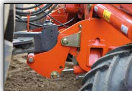
Optional hydr. frame ballasting kit
