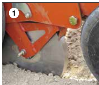
Intermediate heavy stainless steel press wheel
